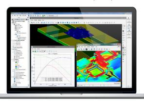
High-frequency components are sensitive to interactions with surrounding PCB traces and vias. These 3D components can be created and simulated in PathWave EM Design (EMPro), and then combined with a board layout in PathWave ADS for complete 3D EM simulation using FEM technology.
